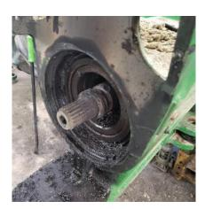
The male component of the gudgeon and the housing – no damage done!
