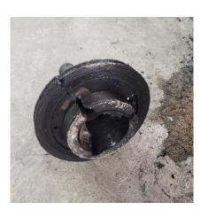
The spindle nut, the female part of the gudgeon - removed
