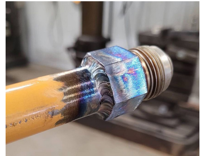
Tartan TIG was used to make this flawless weld on a high-pressure hydraulic application.
