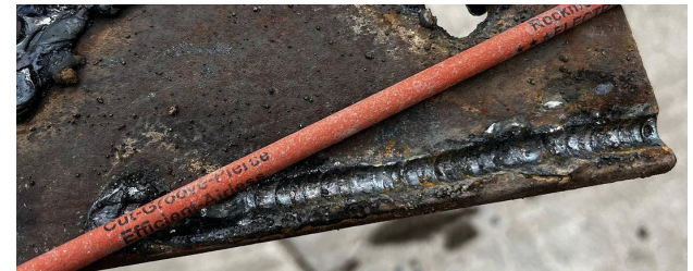
Electra AAA airless gouging rod is a quick way to remove a weld.
